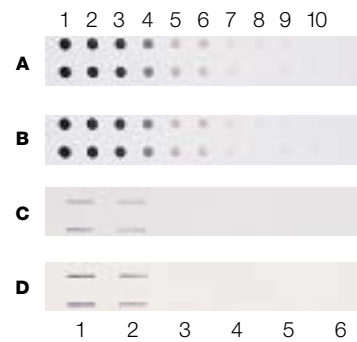
Fig. 2.10. Multiple sample comparisons are simplified with the Bio-Dot and Bio-Dot SF microfiltration units. A and B, antigen (human transferrin) applied to nitrocellulose in each row of the Bio-Dot apparatus. 1, 100 ng; 2, 50 ng; 3, 25 ng; 4, 10 ng; 5, 5 ng; 6, 2.5 ng; 7, 1 ng; 8, 0.5 ng; 9, 0.25 ng; 10, 1% BSA in TBS. C and D, antigen applied to each row of the Bio-Dot SF apparatus. 1, 100 ng; 2, 50 ng; 3, 10 ng; 4, 5 ng; 5, 1 ng; 6, 0.1 ng. The membranes were incubated with rabbit anti-human transferrin. In A and C, Bio-Rad's goat anti-rabbit gold conjugate and gold enhancement kit were used to visualize the antigen. In B and D, Bio-Rad's goat anti-rabbit AP conjugate and the color development reagents BCIP and NBT were used to visualize the antigen.
